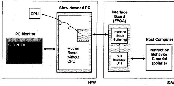
Fig. 3. H/W and S/W co-simulation environment called CMV for the verification of C model
