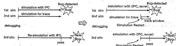
Fig. 12. Reduction of simulation time by the save-and-restart feature of StreC
