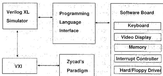
Fig. 6. Gate-level Verilog simulation with Zycad acceleration
