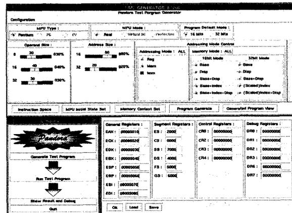
Fig. 9. ATPG(Automatic Test Program Generator) called *Pandora* generates more than 300 test programs with the biasing information of instruction and operand type
