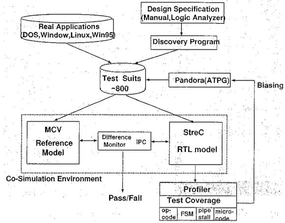
Fig. 11. Test coverage metrics are fed back to the automatic test program generator for more complete test.
