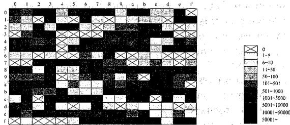
Fig. 10. Number of occurrences of each of 256 instructions in running DOS applications. It is shown that some instructions denoted by a 'cross' were not invoked at all (after 2 million instructions)
