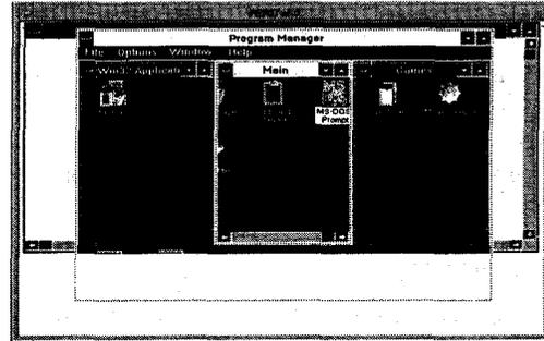
Fig. 15. Screen image showing the successful booting of Windows 3.1 using StreC, which took 48 hours running about 20 million instructions.
