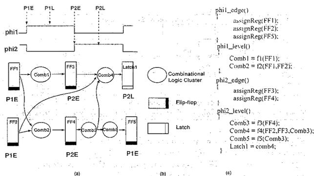
Fig. 5. (a) Signal Flow Graph showing the clock timing of flip-flops(FF's) and latches, (b) symbols for SFG and (c) the corresponding RTL C description, 2-phase clocking scheme was assumed. (In cycle-based simulation, phi1 is simply assumed to be the complement of phi2)
