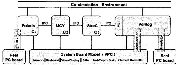
Fig. 4. Co-simulation environment for different design models (i.e., Polaris, MCV, StreC and Verilog) with VPC(Virtual PC). IPC dynamically checks the consistency between models during the simulation
